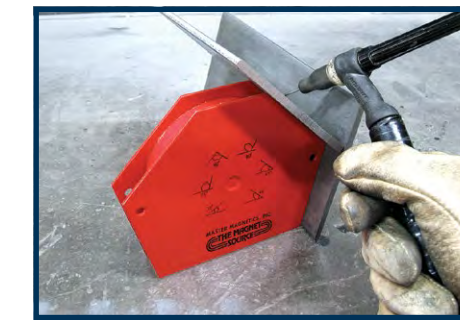
Protractor: for 30, 45, 60, 75 and 90 degree angles
